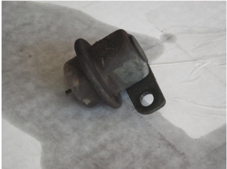
10. Insert the new part into the fuel rail and fasten with the two bolts.
