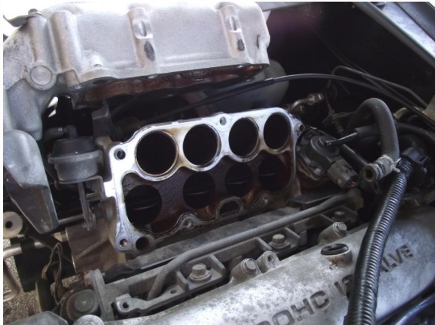
5. Stuff clean rags into the intake ports to ensure you don't drop any small parts into the intake!
