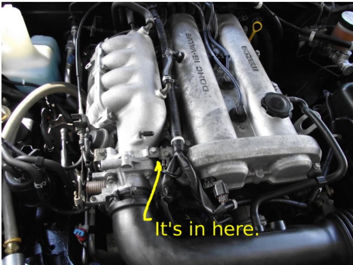
The part is called a *Fuel Pulsation Damper*, and is the second of two. The other is located in an easily accessible place on the passenger side of the chassis under the hood. This is the story of how to replace **Fuel Pulsation Damper #2**.
