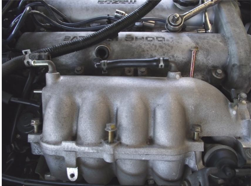
4. Lift the plenum up to clear the alignment pins and tilt the plenum clear of the intake manifold. Note the metal gasket – handle very carefully or plan to replace it.
