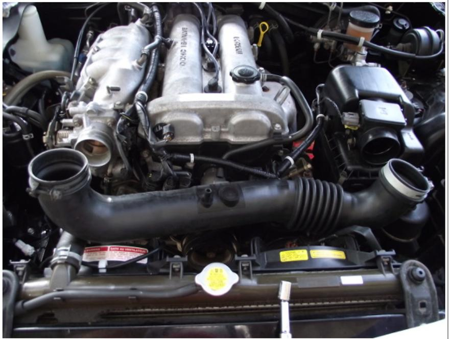
2. Disconnect the numerous electrical connections at the front of the engine, and also the EGR connector at the rear of the intake manifold.
