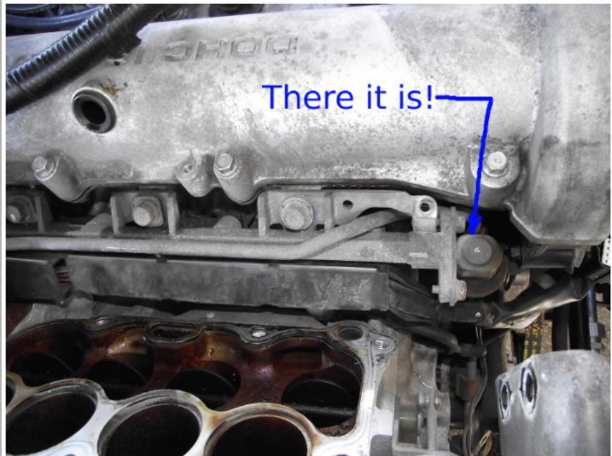
7. Remove the three bolts holding the fuel rail to the cylinder head.
