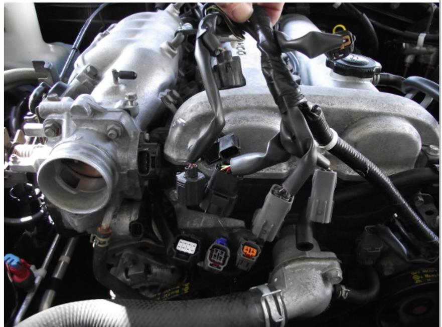
3. Remove the bolts holding the plenum to the intake manifold. There are six bolts on top, and two at the front under the throttle body. Also remove the several hoses from the connections on the plenum and throttle body. Have a plug to insert into the coolant hose under the throttle body so as not to make a mess.
